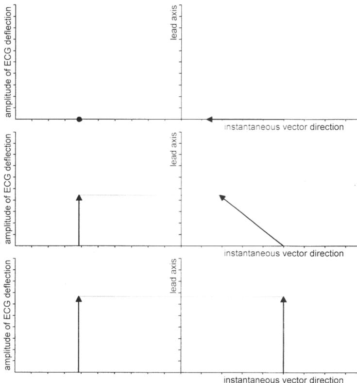
**Fig. 2.** Different amplitudes registered on a lead due to different direction of instantaneous vector.
