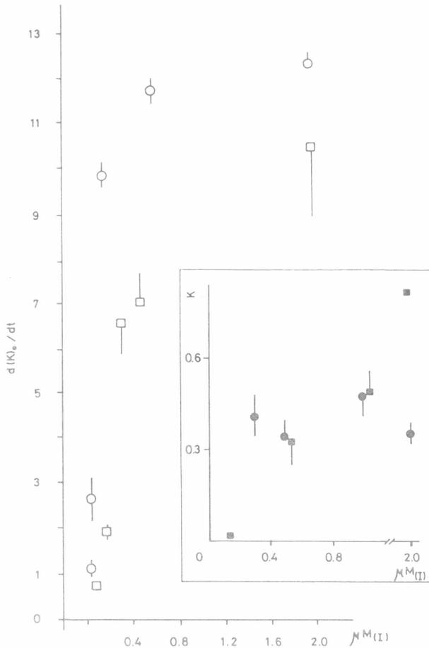
**Fig. 2** Initial rate of potassium loss as a function of the ionophore concentration, in red cell suspensions incubated with A<sub>23187</sub>; aRC (open squares), nRC (open circles). Insert: values of the  $k$  parameter (estimated for different A<sub>23187</sub> concentrations with the first order rate equation as shown in Fig. 1) are presented as a function of the ionophore concentration for aRC (full squares) and nRC (full circles). Vertical bars: S.E.M.
