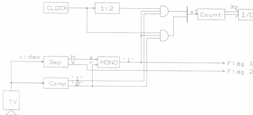
**Fig. 2.** Schematics of the full HW implementation of the simple, single object detection procedure based on evaluation of the videosignal amplitude. The additional HW (compared with the schematics in Fig. 1) consists of: clock, divider (1:2), pair of AND gates, one OR gate and the counter X (Count) with parallel I/O. The additional HW functions correspond to that of the SW described in Fig 1.
