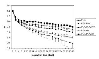
**Fig. 6.** Time-dependent acidification of scaffolds from PGA mixtures.
