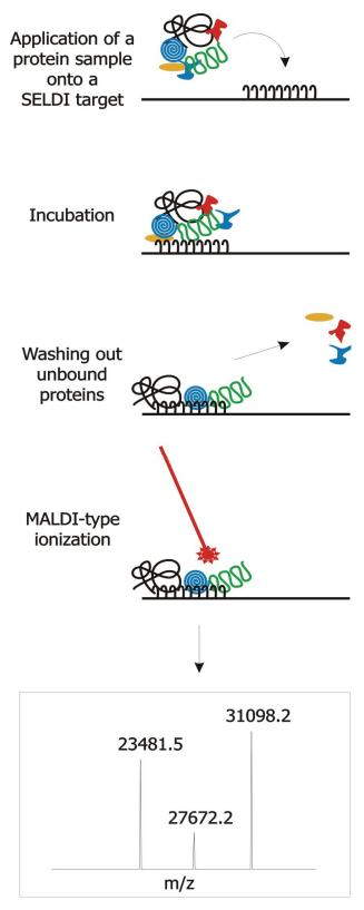
**Fig. 2B.** Protein profiling workflow: Crude sample is applied onto a SELDI target modified by a specific chromatographic surface. After incubation the unbound fraction is washed away. The SELDI chip is directly analyzed using a SELDI-TOF mass spectrometer. A protein profile is obtained, each protein being represented by a peak with a corresponding m/z value. Note that information on protein identity is missing and cannot be obtained by this type of analysis.
