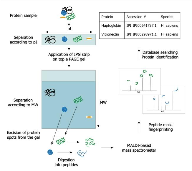
**Fig. 2A.** 2D-PAGE workflow: A complex protein sample is applied onto an IPG strip and the proteins are separated according to their pI. Then, the strip is placed on top a SDS-PAGE gel and the proteins are separated according to their molecular weight (MW) in second, perpendicular dimension. After gel staining, protein spots of interest may be cut out, digested into peptides and identified mostly by means of PMF approach.
