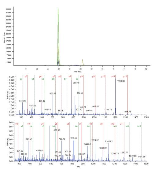
Fig. 7. MRM triggered MSMS. confident MRM should validated be confirming the identity of the chromatographic MRM peaks by additional acquisition of a MSMS spectrum. The MRM trace shows two chromatographic peaks, each eluting at a different time point. a MRM-triggered acquiring MSMS spectrum, the targeted earlier eluting signature peptide is unambiguously identified (upper MSMS spectrum), whereas the second peak (lower MSMS spectrum) was proved to originate from a different protein.
