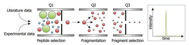
**Fig. 6.** Multiple Reaction Monitoring scheme. Mass spectrometers used for MRM are set to select only a specific precursor peptide in the first quadrupole (Q1), which is then fragmented in the collision cell (Q2), a specific fragment is selected in the third quadrupole (Q3) and detected. The intensity of the Q3 fragment is then plotted in time, which results in a chromatographic peak correlating with peptide amount in the sample.
