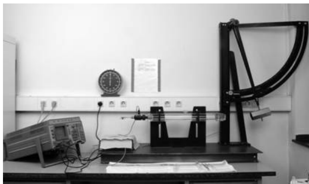
Fig. 1. The fluid percussion model.
