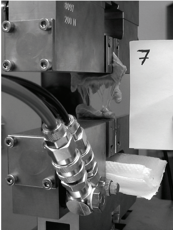
Fig. 1. Heart valve tissue sample between the pneumatic grips of the 200 N loading cell of the experimental apparatus Zwick Roell Z050.
