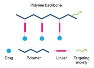
**Fig. 1.** The scheme of the polymer conjugate with the drug and targeting moiety (modified from (Natfji *et al.* 2017)).
