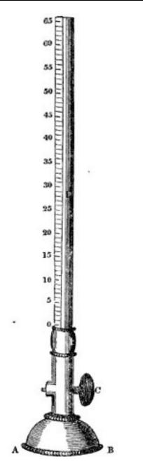
Fig. 1a. Herisson's sphygmometer [9].
