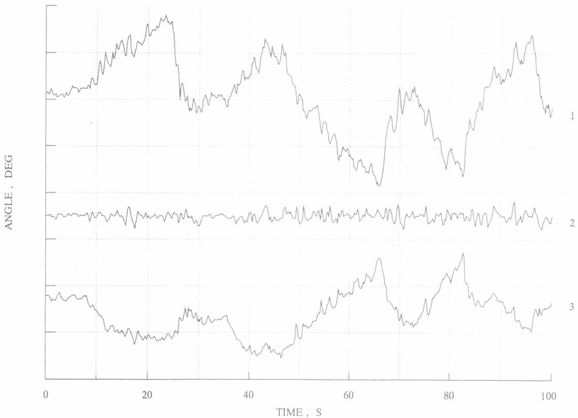
**Fig. 4** The slow voluntary flexion and extension in hip joint on immobile platform. The subject was instructed to maintain the constant angle of shin inclination relative to platform using visual feedback via oscilloscope. 1 – stabilogram, 2 – the angle of shin inclination, 3 – the ankle angle calculated on the basis of the changes of projective length of the soleus muscle. One scale division corresponds to 10 Nm for curve 1 and to 1 deg for curves 2 and 3.
