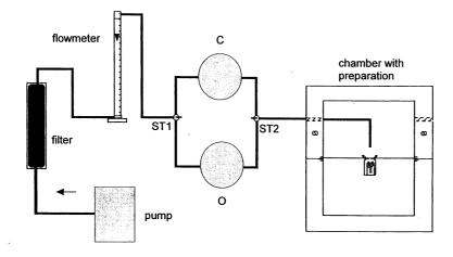
Fig 1. System for application of odors in the neurophysiological experiments. C – chamber with control (water); O –chamber with odor source; SI, S2: stopcocks; the arrow marks the direction of the air stream.
