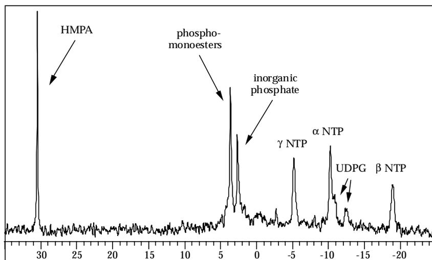
**Fig. 4.** Typical  $^{31}\text{P}$  A549 cell spectrum showing HMPA reference at 30.5 ppm. This spectrum represents a sum of 10 data sets 128 averages each (3 second recycle time) for a total of ~1 hour acquisition. The FID was preconditioned with 10 Hz of Lorentzian broadening prior to Fourier transform. Phosphorous linewidth on HMPA was ~6 Hz.
