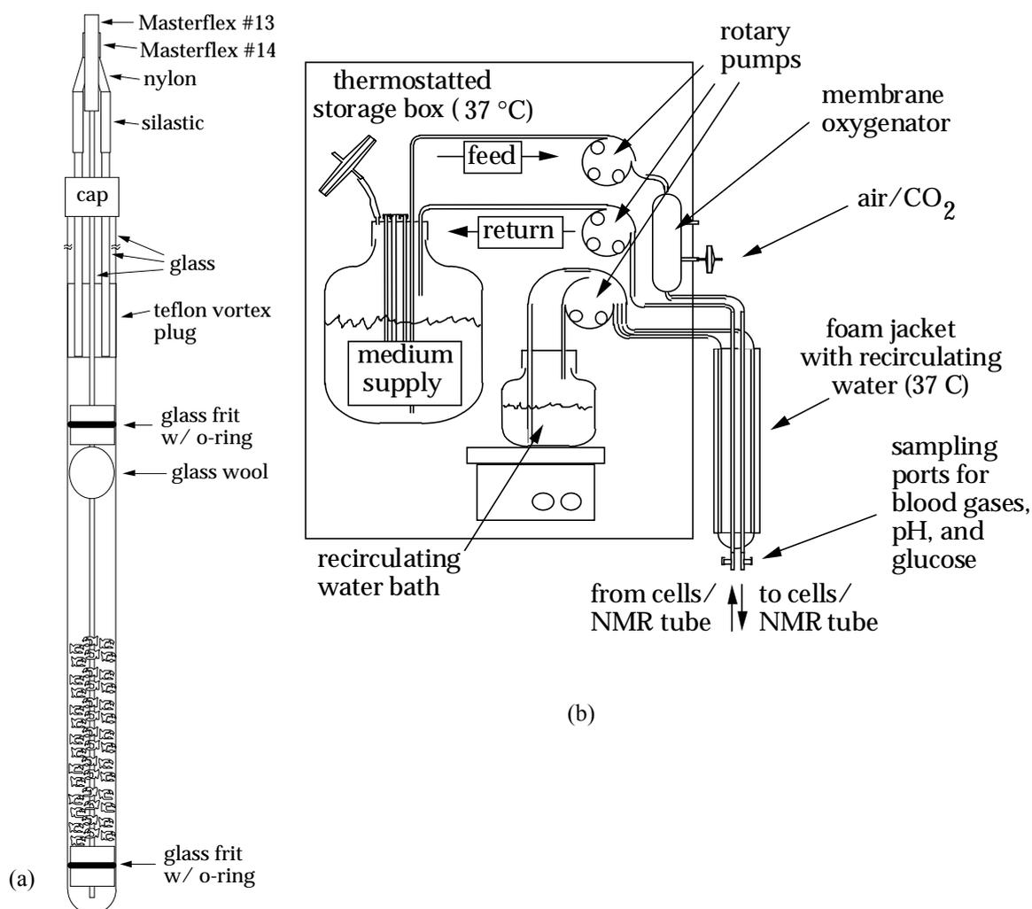
**Fig. 1.** Schematic diagram of a) NMR perfusion chamber and b) perfusion system.
