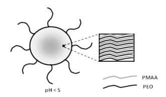
Fig. 3. Presumed structure of hydrogen-bonded nanoparticles.
