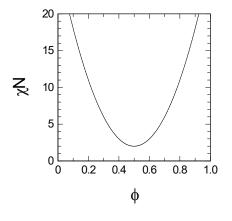
**Fig. 1.** A schematic phase diagram for a polymer A/polymer B or polymer/solvent.  $\phi$  is the volume fraction of the first component of the system, N the number of monomeric units in the polymer chain and  $\chi$  the interaction parameter describing the strength of interaction between polymer A and B or between the polymer and solvent.
