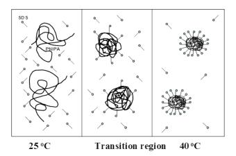
**Fig. 2.** Schematic representation of nanoparticle formation by precipitation of PNIPAM when heated above the LCST and by interaction with surfactant molecules of SDS.
