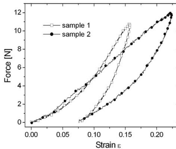
**Fig. 3.** Examples of loading curves for intact hyaline cartilage tissue from non-weight-bearing zone (sample 1) and cartilage from the defect zone (sample 2). Preload of 1N was considered.
