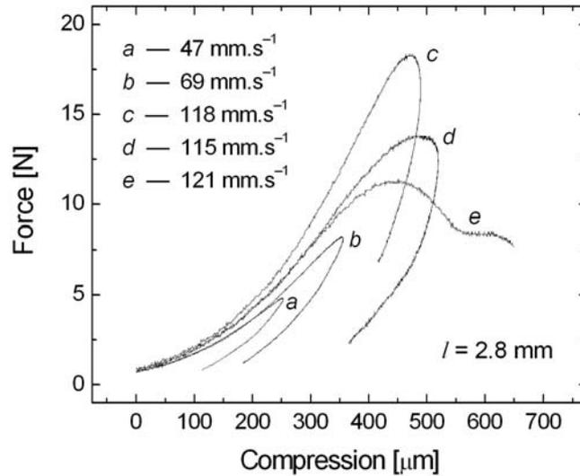
**Fig. 4.** Force-compression loading curves of single hyaline joint cartilage sample - consequent measurements a to e taken in intervals of 5–10 s. The initial impact velocities  $v_i$  are denoted for each measurement. Uncompressed sample thickness  $l = 2.8$  mm.
