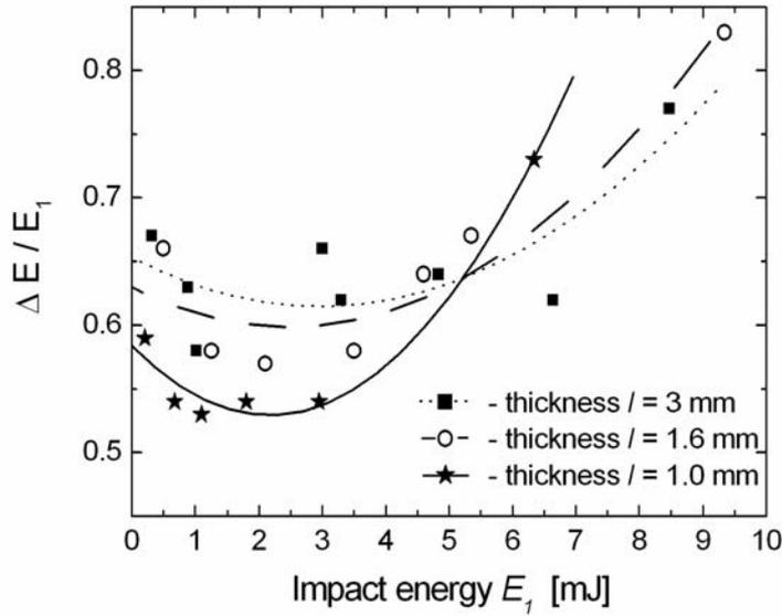
**Fig. 6.** Dissipation of the impact energy vs. overall impactor energy for three native cartilage specimens. Quadratic fit is shown for each sample data set. Thickness  $l$  of individual samples is denoted.
