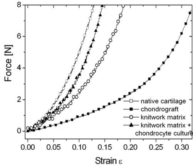
**Fig. 7.** Loading curves of native cartilage and some of the materials tested: native cartilage sample (the same as in Fig. 2), fibrin chondrograft used for autologous chondrocyte transplantations, knitted chirlac fiber matrix – blank damped in physiological solution and the same chondrocyte-seeded matrix after a ten-day cultivation.
