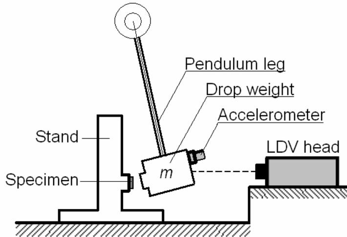
**Fig. 1.** Scheme of impact loading measurement setup.
