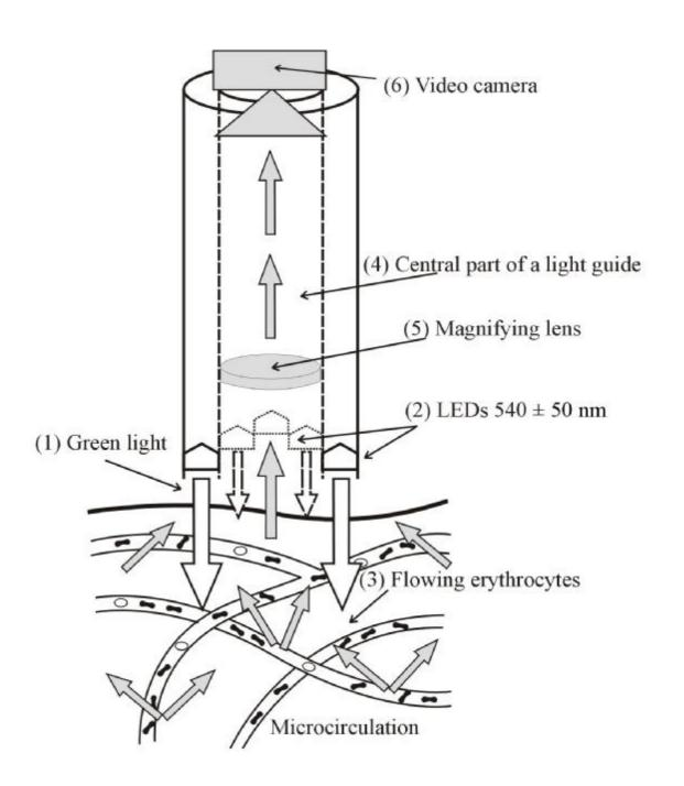
Figure 2 – A scheme of the stabilizing and fixation device for SDF imaging probe
