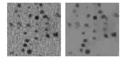
Image of silver nanoparticles (Silver proteinate, Fluka, Switzerland) before  $TV - \mathbf{L}^1$  regularization and after it. Transmission electron microscopy images were provided by Anatolij Filimoněnko from IMG ASCR. Even the less contrast objects were preserved by the filtration and the resulting image is suitable for further processing and detection of particles by adaptive thresholding.
